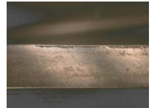
逃げ面 Relief face /逃げ面摩耗量0.09mm Flank wear
